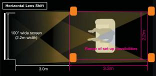
The projection screen can be moved left or right nearly 2 screen widths. 'The horizontal lens shift allows the center of the screen to be shifted approximately half a screen width to the left or right of center.
