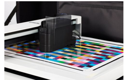
Automatic media thickness and position detection
