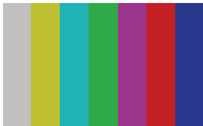
Colour Bars To check the colour appearance, colour reproduction and colour bleeding
